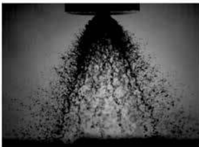
Shadowgraph image of Pintle Injector Spray
