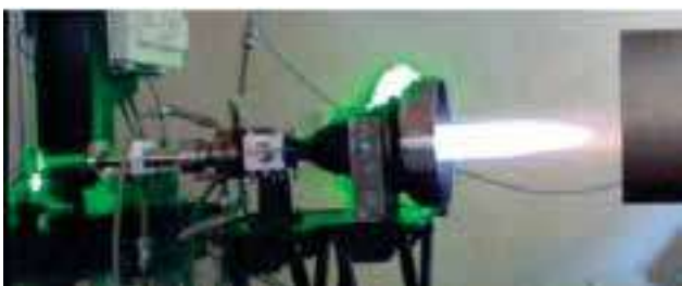
Laser Ignition System developed at IIST
