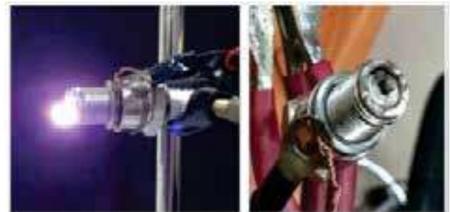
Surface discharge spark plugs developed at IIST
