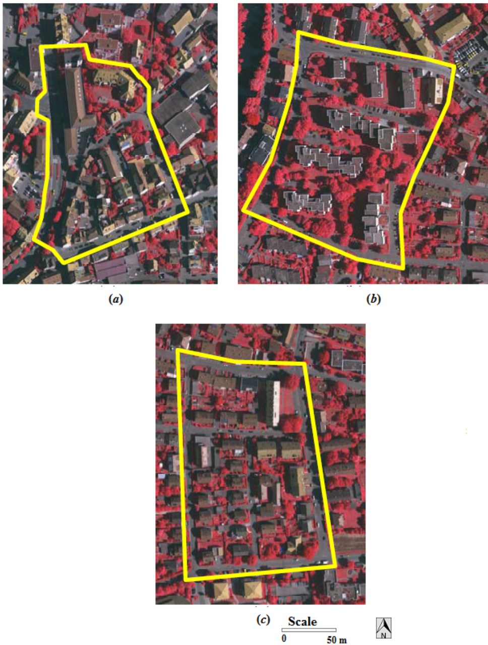
Figure 3.1: Aerial photographs of the study area with NIR band mapped to red, red band mapped to green and green band mapped to blue to create a false colour composite (a) study area 1 : inner city, (b) study area 2 : high riser, (c) study area 3: residential area
