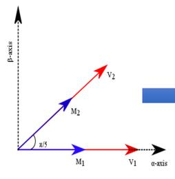
Fig.4: Large and medium voltage space vectors in sector-1 of  $\alpha$ - $\beta$  plane
