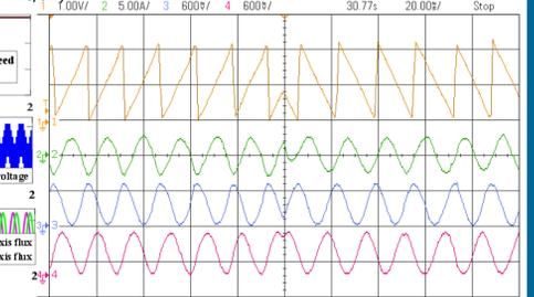
Fig.14 Experimental result during speed reversal: 1. Stator flux angle (Y axis 3.14rad/div), (X axis 20.0 ms/div) 2. Phase-A current (Y axis 5A/div), 3. Alpha-axis stator flux,(X axis 20.0 ms/div) 4. Beta-axis stator flux,(X axis 20.0 ms/div).
