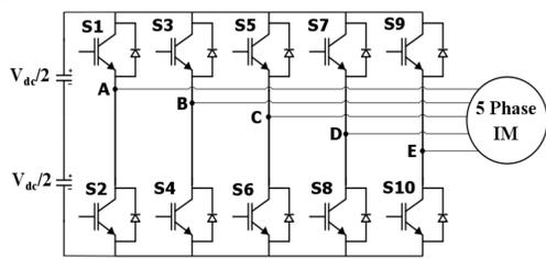
Fig.1: Five-phase VSI fed Induction Motor
