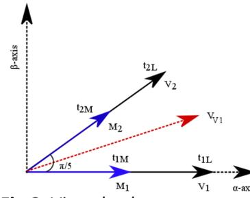
Fig.8: Virtual voltage space vector and corresponding large and medium space vectors in  $\alpha$ - $\beta$  plane
