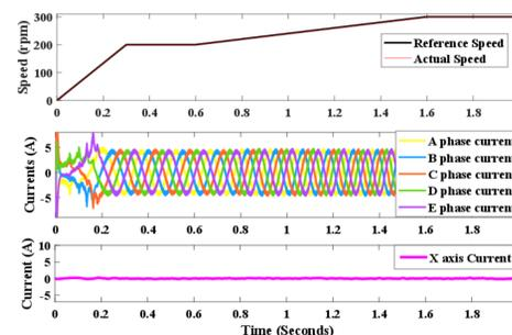
Fig.11 Simulation results of loaded condition: 1. Actual speed and reference speed(rpm) (b) Five stator phase current (c) X-axis current
