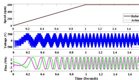
Fig.12 Simulation results during no load operation: 1. Actual speed and reference speed(rpm) 2. Phase voltage (Volts) 3. Flux (Weber)
