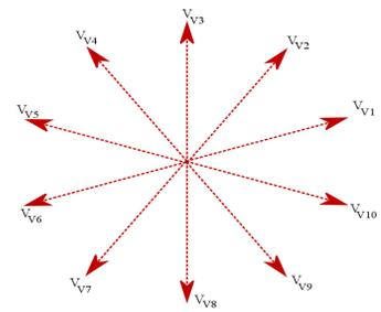
Fig.7: Virtual voltage space vectors in 5-phase VSI
