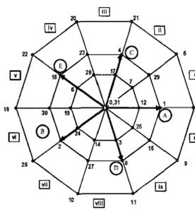
Fig.3: Space vector diagram in  $x$ - $y$  plane
