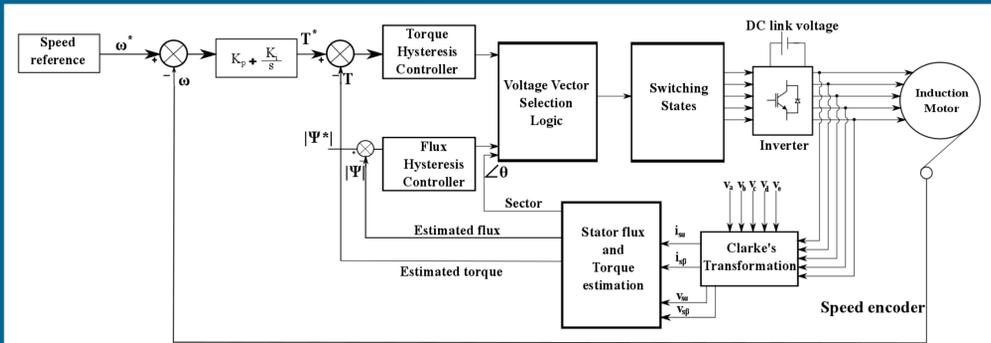
Fig.10 Block diagram of direct torque control of five-phase induction motor
