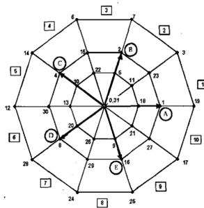
Fig.2: Space vector diagram in  $\alpha$ - $\beta$  plane
