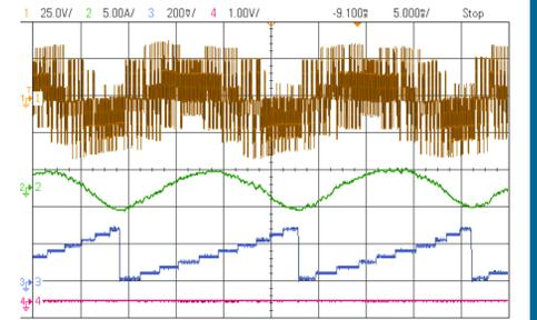
Fig.13 Steady state experimental result : 1. Phase-A Voltage (Y axis 25V/div), 2. Phase-A Current (Y axis 5A/div), 3. Sector information (0-10), (X axis 5.0 Ms/div) 4. Stator X-axis Average Voltage(Y axis 1V/div),(X axis 5.0 Ms/div).
