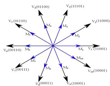
Fig.6: Actual large and medium voltage space vectors in 5- phase VSI
